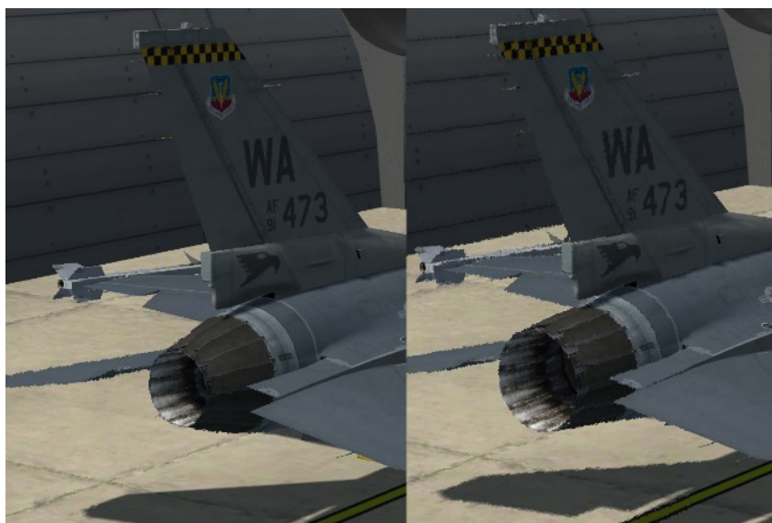
Performing the SEC check, nozzle closing & opening
