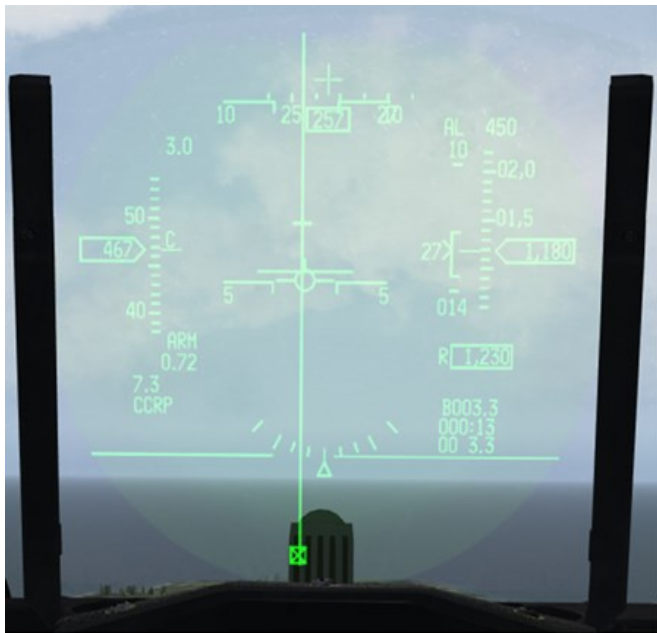
Initiate pull and keep FPM on VSC Timer reset to time to release
