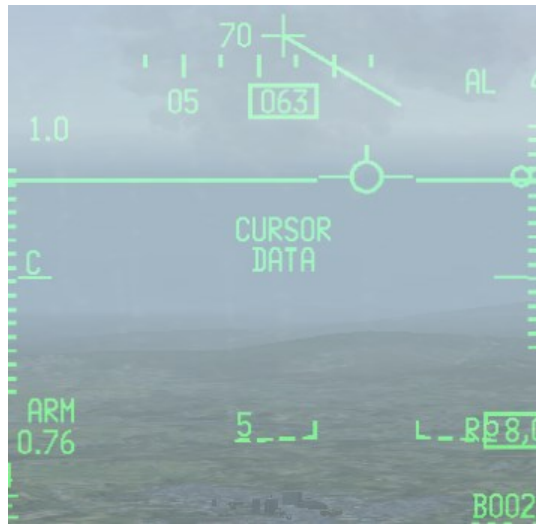
Assignee (#3's) FCR, HSD and HUD. Assigner (#1) sent cursor data NNE of ownship Markpoint
